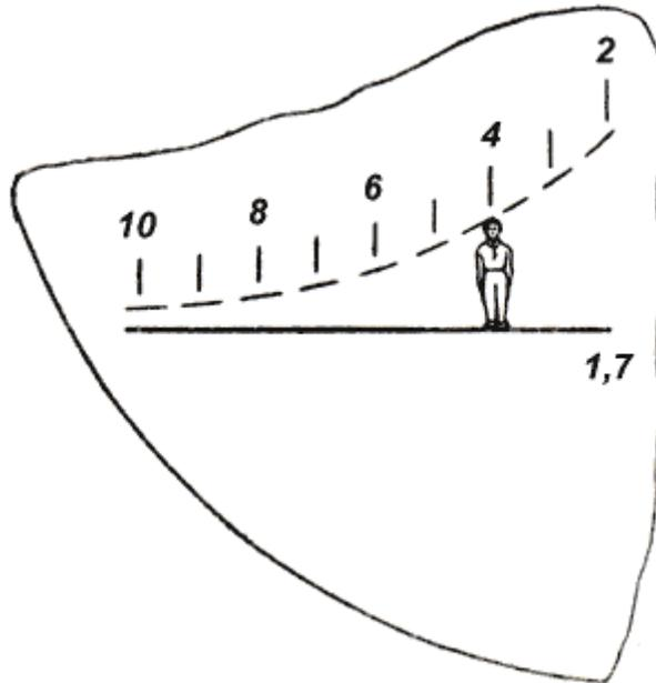
**Fig. 13. Range-finding scale**
